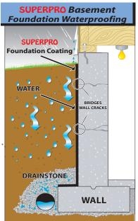
Good building practices for foundation backfill material referenced by the National Building Code. Soils that contain sharp angular stone and glacial til clay require the addition of a protection board or drainage mat such as **SUPERDRAIN** 5200 or **SUPERSEAL** Dimpled Foundation Membrane or equivalent
